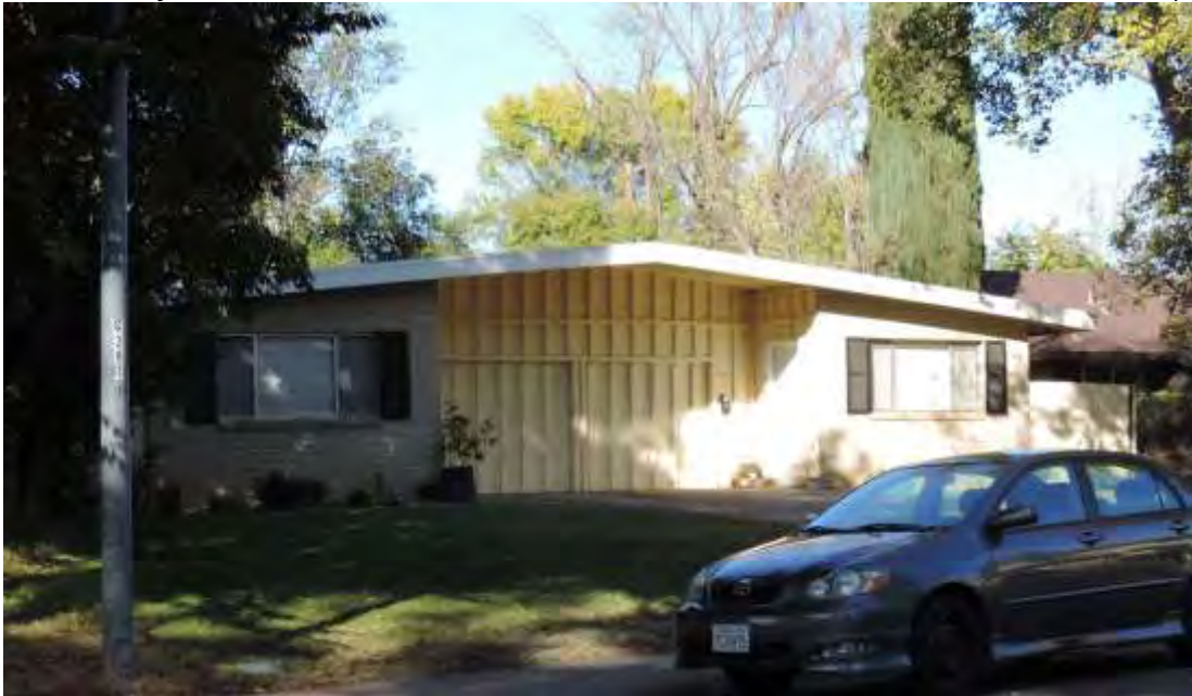
Photograph 8: 25 – 27 Simmons Way, Example of anomalous front-gabled Post-and-Beam duplex with double single garages, board-and-batten cladding, and brick accents.
